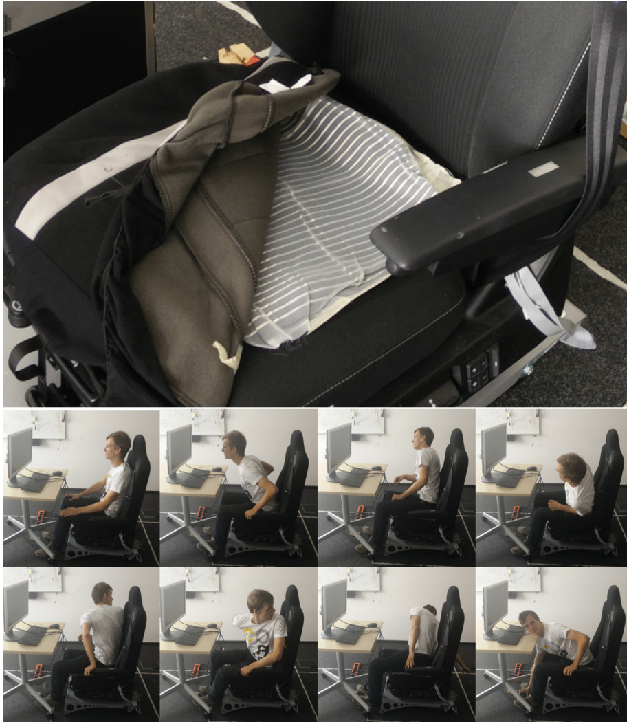
Fig. 5. The textile pressure matrix as a seat cover. Postures from top left to bottom right: sit normal, lean front, lean right, lean left, look back right, look back left, reach back right and touch floor.
