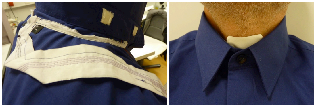
Figure 9 the 2 nd sensor shirt: sensors and their conductive yarn wiring under the collar (left) and sensor outlook (right)
